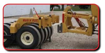
The Walk 'n' Roll Heavy Duty Lift Assembly attaches to the motor grader like a factory rear ripper. It uses the same bolt pattern so there is no welding or holes to drill to mount the lift assembly. The lift assembly requires an extra valve and hydraulics to the rear of the motor grader. Parallel lift raises and lowers the front and rear tires simultaneously assuring equal pressure on all of the tires.
