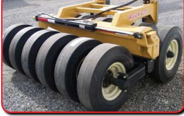
The unit shown is the WR90RL. This unit will Side-Shift 24" to the Right or Left. We also build a WR75R and a WR90R Hydra-Slide. These units Side-Shift 36" to the Right
