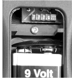
Figure 7: DIP Switch in Remote Handset Battery Compartment
