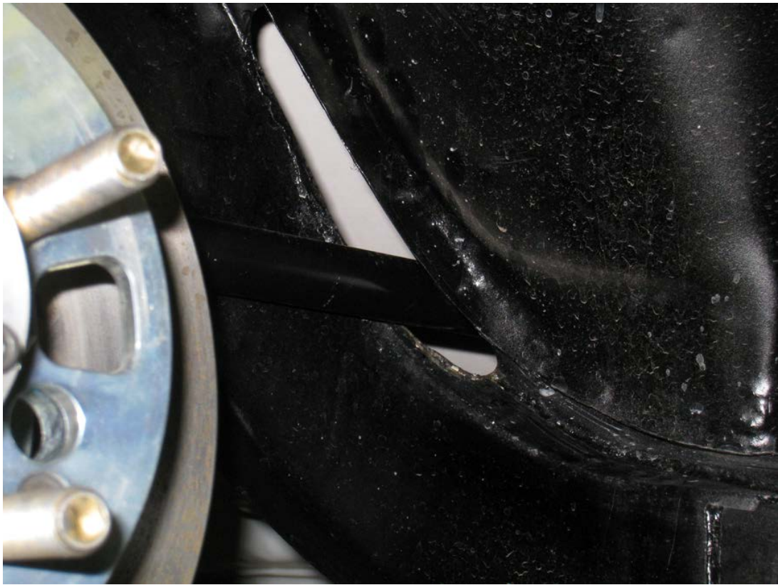
An outside view showing slot location next to frame and vertical relative to override bar with hanging suspension.
